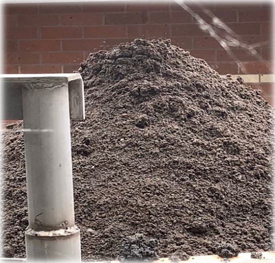
3. Much dryer cake with the liquid polymer.
