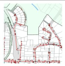
This project replaces 4015 feet of 8-inch cast iron pipe with 8 and 12-inch ductile iron pipe. It will also create a loop in the system where the District has had to flush more often to keep the water fresh tasting.
