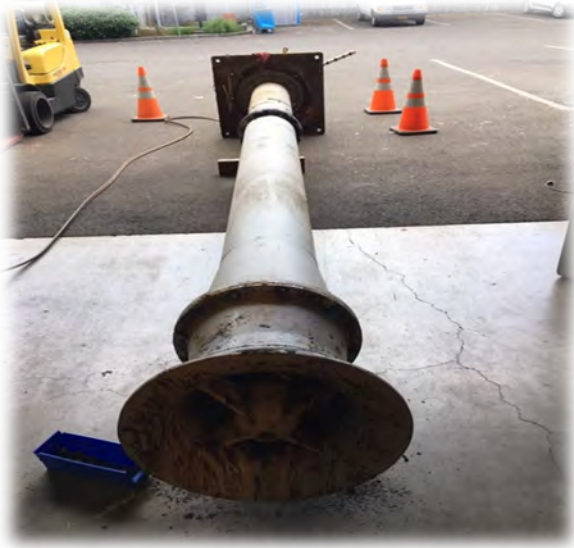
1) Suction bell end of MLR pump
