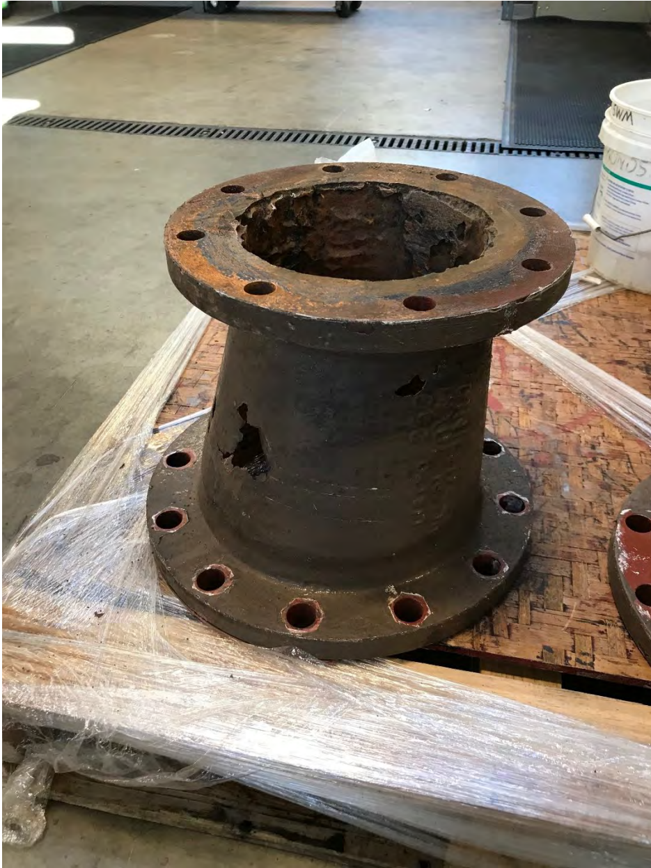
Photo 2 The corroded cone from Digester Mixing Pump #2. When you are pumping liquids, this is not something you want to see.
