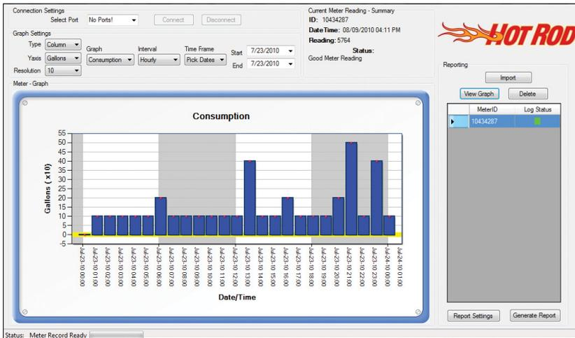
**24-Hour Consumption Graph** – Graph display shows where usage does not go to zero during any 24-hour period, identifying a possible leak.
