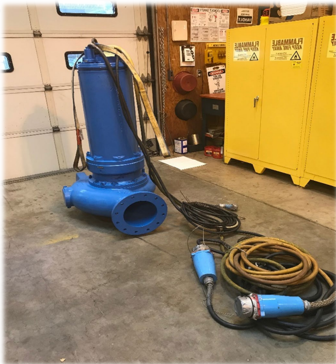
Influent Pump finally rebuilt and returned
