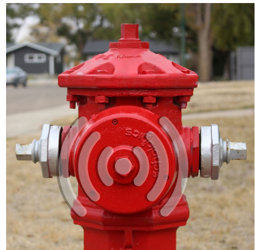
Battery-powered monitoring “nodes” incorporating an ultra-sensitive acoustic sensor built into fire hydrant pumper nozzle caps enable the system to identify and locate potential leaks or flow issues.
