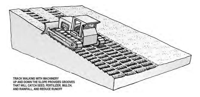
Leaving the slopes in a roughened condition after clearing or creating a rough soil surface with horizontal depressions or grooves will trap seed and reduce runoff velocity. Roughening can be accomplished by 'track walking' slopes with tracked equipment, by using a serrated wing blade attached to the side of a bulldozer, or by other agricultural equipment.
