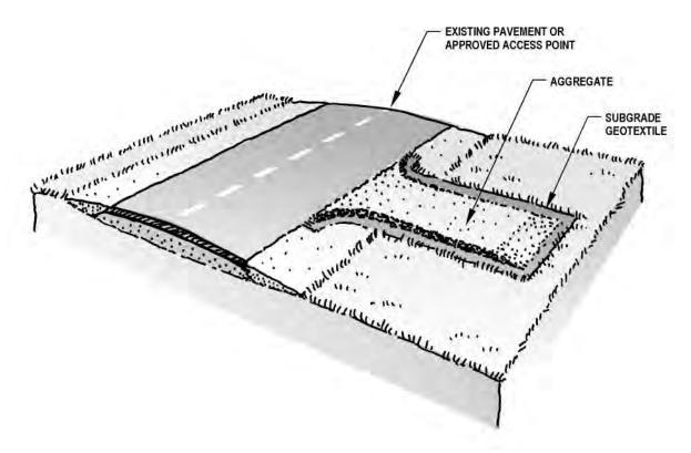
A stabilized rock pad, placed at construction site ingress/egress locations, that reduces the amount of sediment transported onto paved roads by vehicles or runoff. The Construction Entrance also includes a curb ramp designed out of wood.
