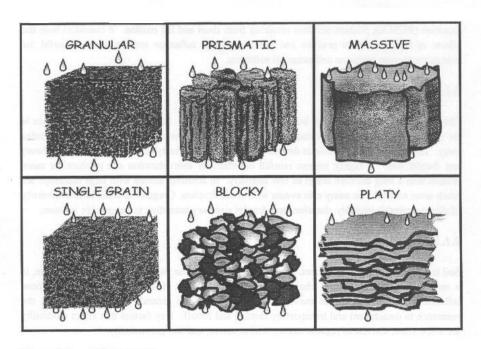
Figure 2-3 Soil Structure
