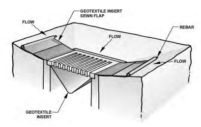
Inlet Protection - Prefabricated Filter Insert
