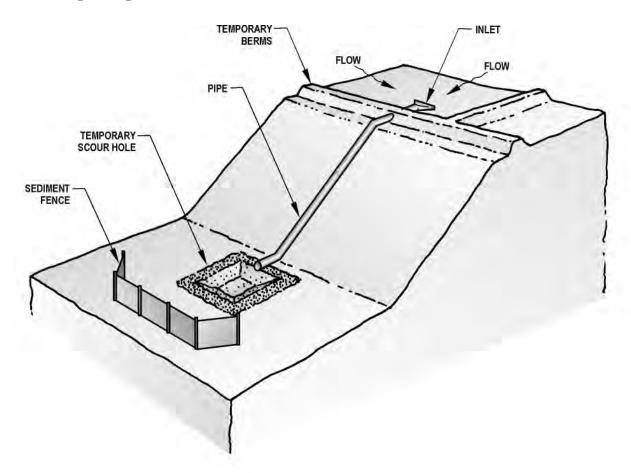
A pipe extending from the top to the bottom of a cut or fill and discharging into a stabilized watercourse, sediment trapping device or onto a stabilized area. The pipe slope drain carries concentrated runoff down steep slopes without causing gullies, erosion, or saturation of slide-prone soils.
