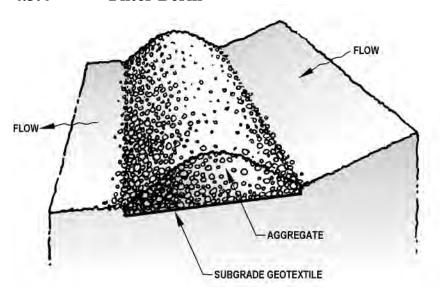
**AGGREGATE BERM** - Retains sediment in gravel or crushed rock berm.
