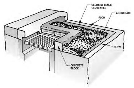
Inlet Protection – Masonry / Aggregate
