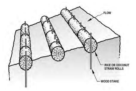
Wattles are manufactured from straw, coconut, or other material that is wrapped in tubular plastic netting. They are approximately 8-9 in. diameter by 7-25 ft. long. Wattles are placed in shallow trenches and staked along the contour of newly constructed or disturbed slopes.
