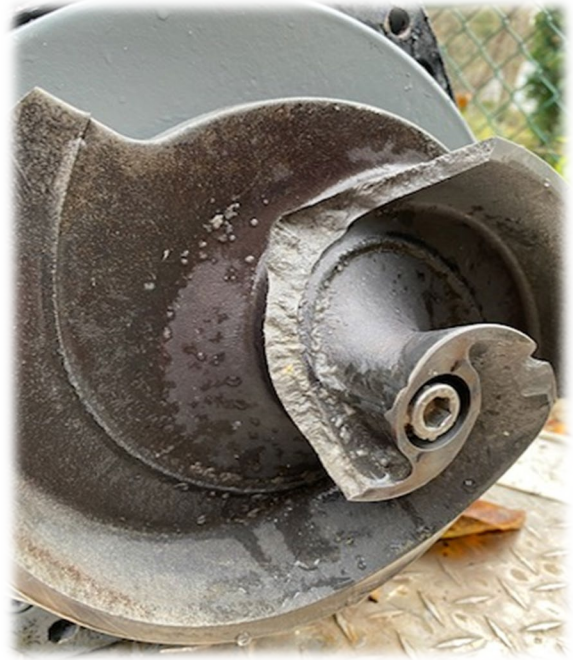
Another Angle of the Broken Impeller.
